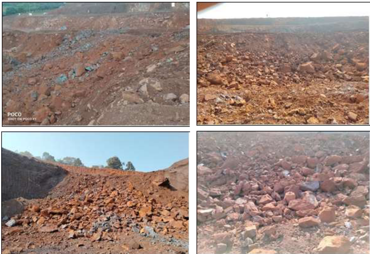
Figure -7: Blasted muck piles (4 Nos)
